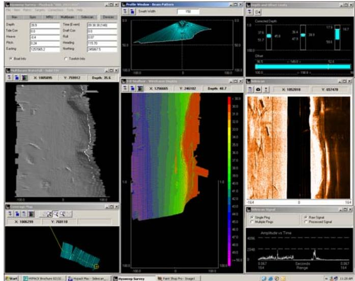
**HYSWEEP® SURVEY:** The data collection program of **HYSWEEP®** runs simultaneously with the SURVEY program of **HYPACK®**. It provides real time display, QC functions and data logging for most commercially available multibeam systems, including those from Atlas, Odom, Reson, Sea Beam and Simrad. A coverage map lets you examine the bottom coverage in real time, ensuring that you have 100% or 200% coverage before leaving the area.
