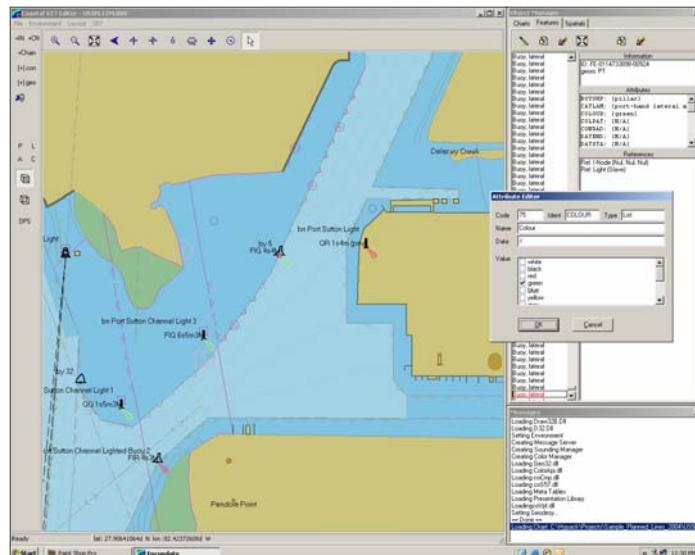
**ENCEdit** is a new HYPACK® module that allows you to create, modify and verify ENC data in S-57 format. ENCEdit provides you with tools to re-attribute, create, move or delete existing features. You can also create new features by manually entering coordinates, by importing data from DXF/DGN, or by transferring targets in real time from SURVEY directly into ENCEdit.
