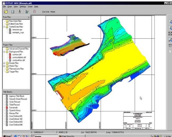
**FINAL PRODUCTS:** The ability to create the final products you need separates **HYPACK®** from the rest. The plotting program generates professional smooth sheets with soundings, grids, graphics and contours in a WYSIWYG display. The VOLUMES program is the de facto standard of the U.S. Army Corps of Engineers for the computation of quantities in dredging projects. TIN MODEL creates surface models that can be used for contouring, volume computations and surface visualization.
