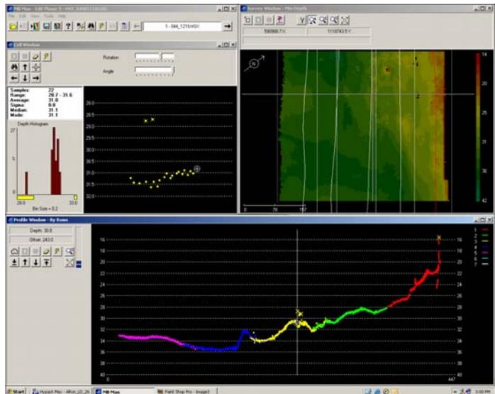
**MULTIBEAM EDITING:** Multibeam data editing, sonar alignment calibration and system performance testing are all provided in the powerful MULTIBEAM EDITOR of **HYSWEEP®**. The program performs automatic or manual filtering, using geometric and statistical methods. It also contains the Performance Test that measures the overall performance of your system versus beam angle as required by USACE. **HYSWEEP®** can also use water level corrections created from RTK GPS elevations.
