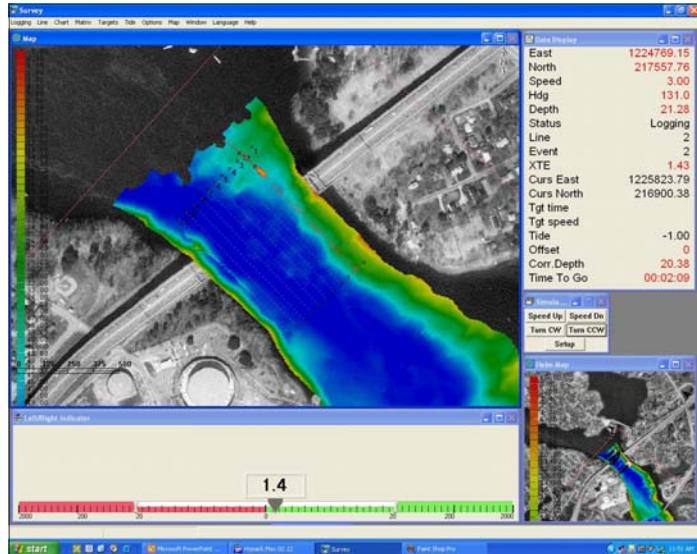
**SURVEY:** **HYPACK®** contains interface drivers to over 200 devices including positioning systems, echosounders, heave-pitch-roll sensors, gyros and other types of equipment. SURVEY supports a single vessel or multiple vessels, along with towfish and ROVs. Data is logged with incredible precision (<1mSec). Survey data and windows can be broadcast over a network to any other computer or saved to a file using our Shared Memory Output routines.
